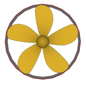
The impeller perimeter shall be the length of the circumference highlighted in red.
